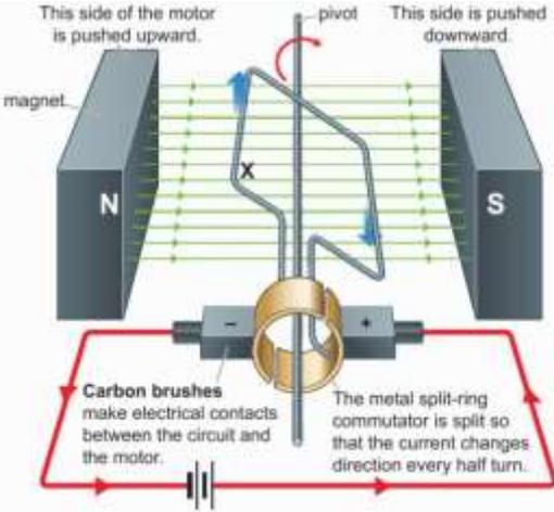
This side of the motor is pushed upward. This side is pushed downward.
