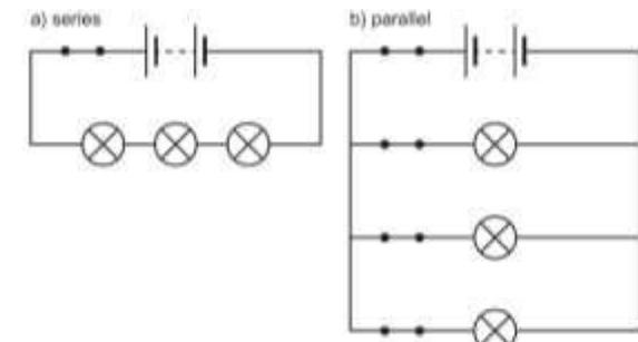
**D** three lamps connected in a) series and b) parallel
