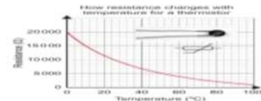
**C** The resistance of a thermistor changes with temperature.
