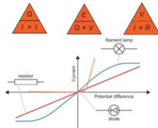
**A** graph of current against potential difference for a fixed resistor, filament lamp and diode
