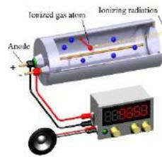
A GM tube can be connected to a counter, to count the pulses of current, or the GM tube may give a click each time radiation is detected. The **count rate** is the number of clicks per second or minute.
