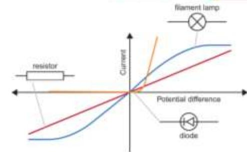
A graph of current against potential difference for a fixed resistor, filament lamp and diode
