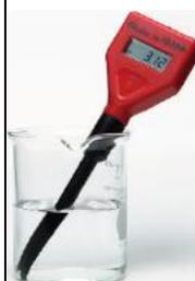
A digital pH meter can give a more accurate value for the pH of a solution. This is because it has a greater **resolution** – meaning it can record pH to a higher degree of accuracy (one or even two decimal places).
